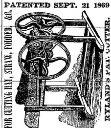
The merits of this machine consists in part, in the attachment of curved knives to the arms of the cutting-wheel, the shearing cut across the mouth-piece, the great power and directness of the blow, by which treble the volume of material is cut, with less power than is required by any other machine; those combined with its durability and simplicity of construction, command public attention. Nothing liable to get out of order, but what a boy could remedy with
