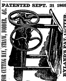
The merits of this machine consists in part, in the attachment of curved knives to the arms of the cutting-wheel, the shear-ing cut across the mouth-piece, the great power and directness of the blow, by which treble the volume of material is cut, with less power than is required by any other machine; those combined with its durability and simplicity of construction, command public attention. Nothing liable to get out of order, but what a boy could remedy with a pocket wrench.
