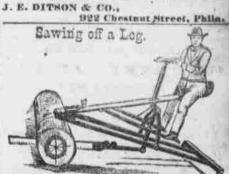
This SAW MACHINE is a wonderful inrention. The weight of the man who is sawing does half of the work. It saws logs of any size, and will saw off a 2 foot log in 2 minutes, Circulars free. Address, Wm. GILES, 696 W. 6th St., Cincinnati, Ohio.
