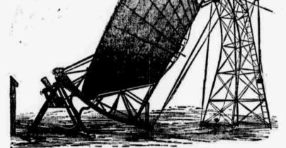
THE SOLAR MOTOR, SIDE VIEW. Showing the Fixed Support and Mounting of Reflector.
