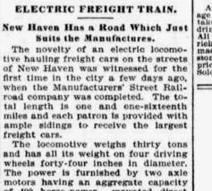
Delightful SPRINC of 400 horse-power, mounted direct without gearing on the axles. The truck, which hangs directly from the ournal boxes, is made of heavy eye beams and carries the motors and cab
