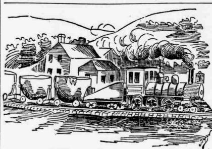
HAULING THE MOLTEN METAL FROM BLAST FURNACES TO OPEN-HEARTH FUR-NACES AT HOMESTEAD.
