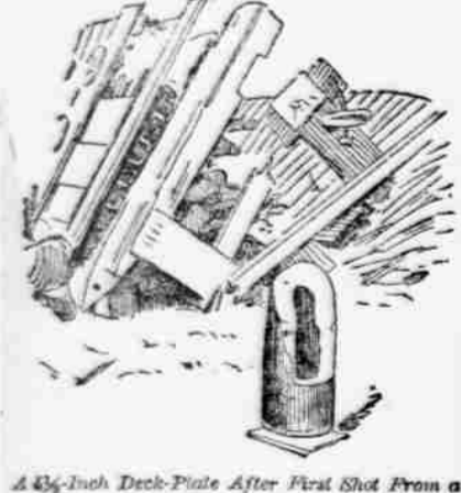
A 4 1/2-Inch Deck-Plate After First Shot From a 12-Inch Mortar.
