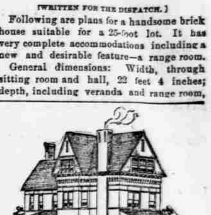
60 feet 4 inches. Heights of stories: Cellar, 8 feet; first story, 9 feet 6 inches; second story, 9 feet; attic, 8 feet.
