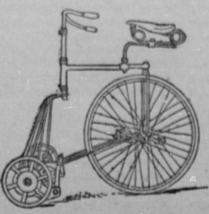
A BICYCLE LAWN MOWEB. hand mower to the hind wheel and trame of an ordinary bicycle. The mower wheels have rubber tires, and the attachments are made by means of steel prongs as shown in the picture. It is said to work three times as fast as an ordinary hand mower.
