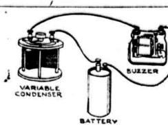
How to test a condenser. The left hand diagram shows how the plater are arranged. There is no electrical connection between the two sets of plates. To the right is the hook-up for testing as explained in the article
