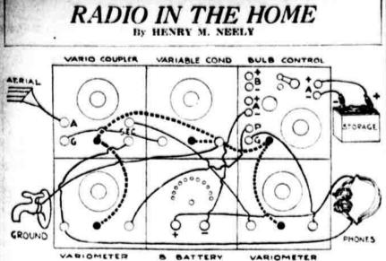
Here's the "short wave regenerative" hook up as used with the "unit" method of building that we have been describing. Six of the units fit together and give the appearance of a complete cabinet. Best of this system is that, if you want to try other hook-ups, it's easy to take apart and put together another way. The dotted line is the wiring of the "body capacity grounds"
