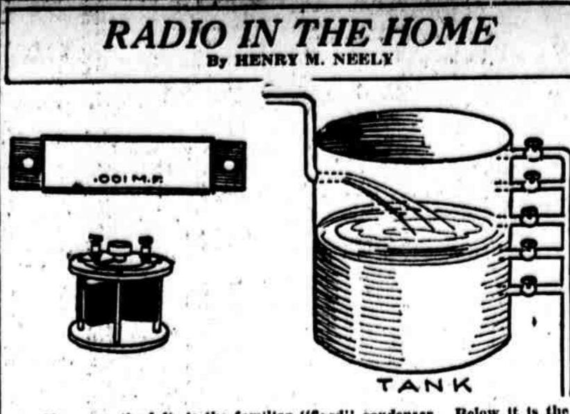
Above, on the left, is the familiar "fixed" condenser. Below it is the more familiar "variable" condenser. To the right is a supposititious water tank by which the accompanying article explains what the two kinds of condenser are and how they work
