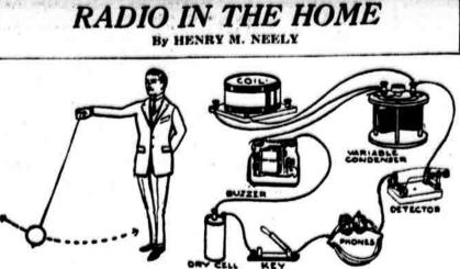
A radio circuit vibrates or swings back and forth just as a pendulum does. The longer the pendulum, the longer arc it makes, and the greater length of time it takes to make a vibration. To the right is a collection of instruments that make vibrations and detect them in a radio circuit. We have means of varying them just as we vary the vibrations of the pendulum. The article explains it
