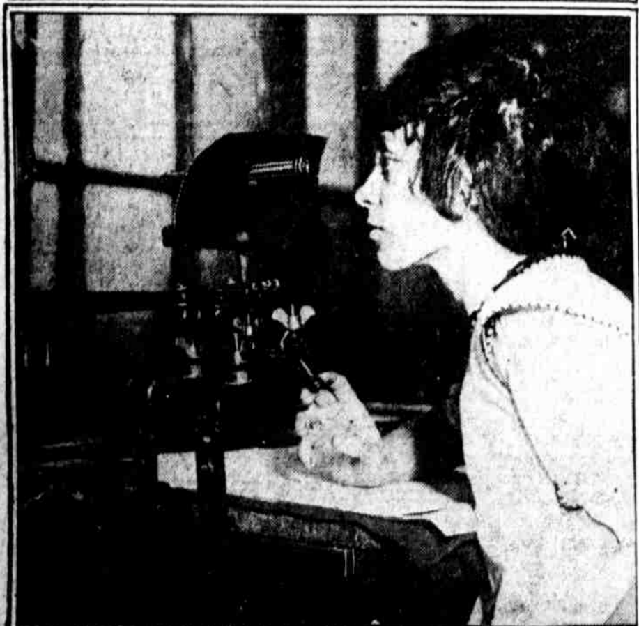
GROUND WIRE OR CROSSED WIRES can be located by telephone companies by means of this instrument, manufactured by Queen-Gray Company, at 16 W. Johnson st. Sophie Dobratski, 62 W. Johnson st. is adjusting it. L. P. S.
