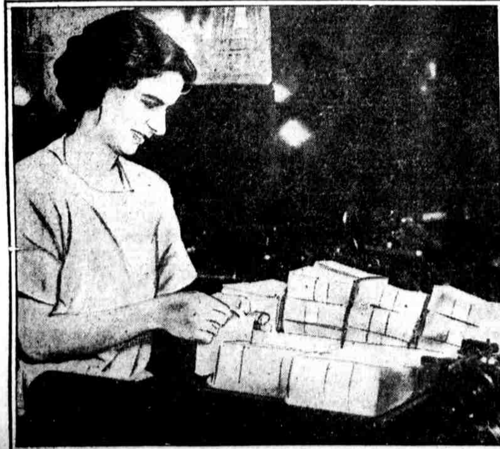
MISS ANNA MCCARTHY, 1612 North Second street, operating a folding machine in an E. J. Spangler Company factory, 1237 North Howard street. The machine throws envelopes in packs of twenty-five; 5000 packs are finished a day. Ledger Photo Service
