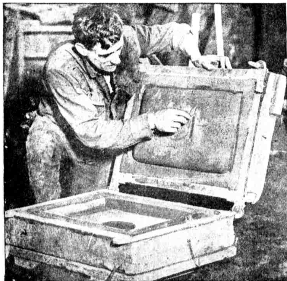
WALTER HOLNQUIST, of 2145 North Orianna street, molding a stove door for the Kappler Fox Foundry Co., in its foundry at 2027 East York street. He can finish thirty-five in a day. Ledger Photo Service.
