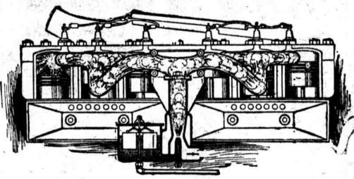
This cross-section of a shows how gasoline that vaporises fast sweeps into the cylin-ders. (Cylinder at ex-treme left exploding.)
