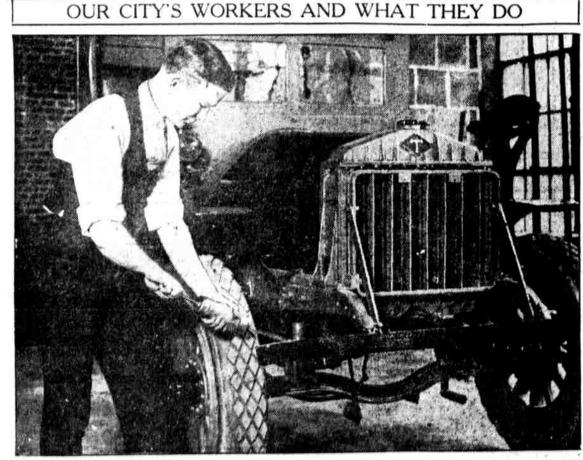
T. J. MOLLOY, 5831 Catharine street, using a lubricating pump on a truck equipped with high-pressure lubricating system at the service station of the Alemite Lubricating Co. of Pennsylvania, 824 North Broad street Ledger Photo Service.
