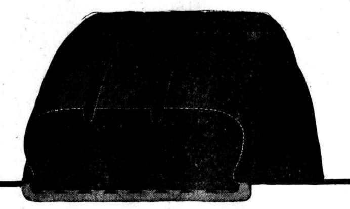
Note the contour of this cross section—the extra amount of rubber, width of tread. This gives broader road contact, giving more effective traction, greater cushioning to the load and longer life for tire and truck.
