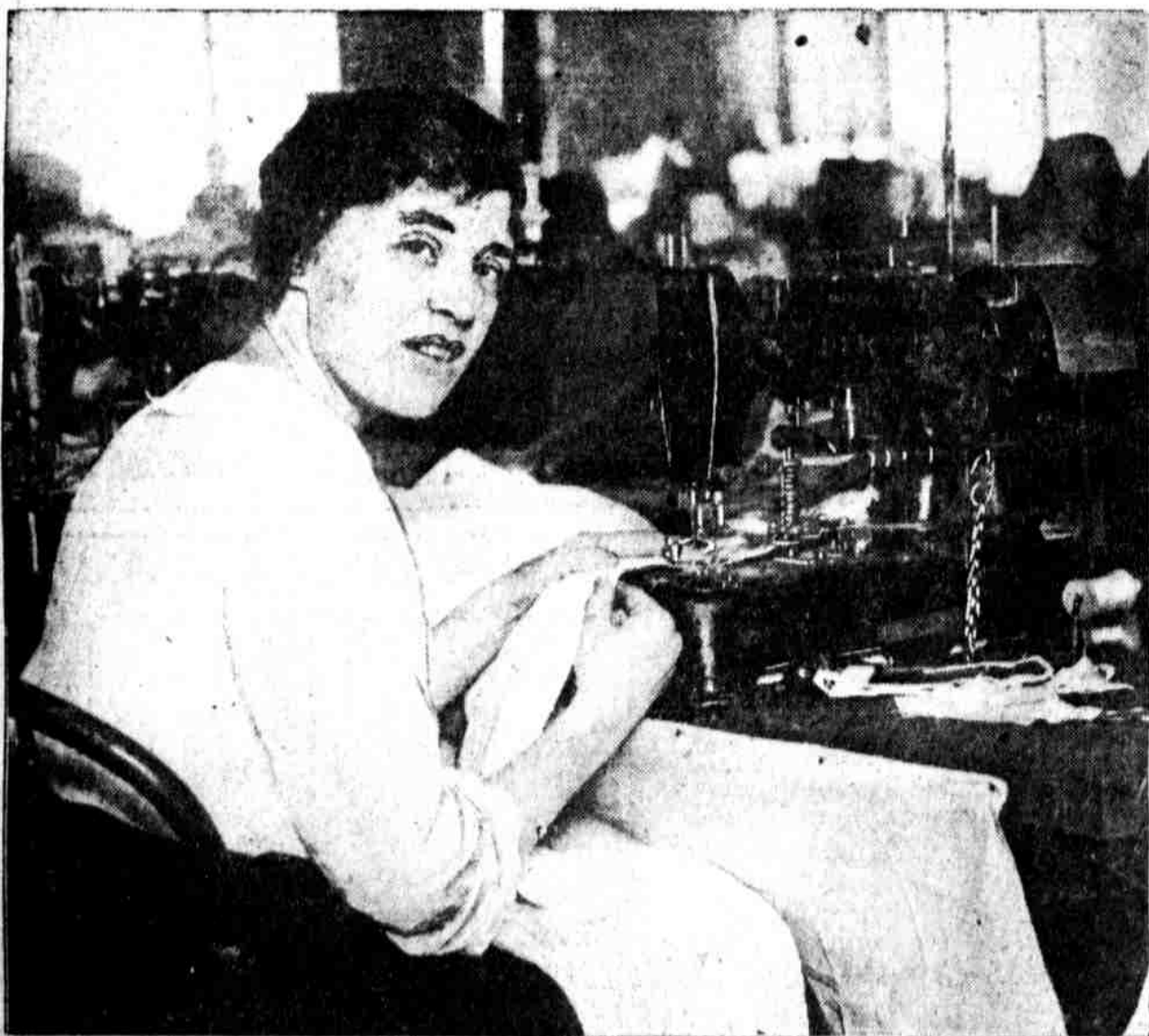
MISS MARY DOUGHERTY, 1607 Federal street, operating a machine for Charles E. Shedaker & Sons, Sixth and Filbert streets, that cuts and sews buttonholes in shirts. Eighty dozen shirts are run through this machine in a day.
