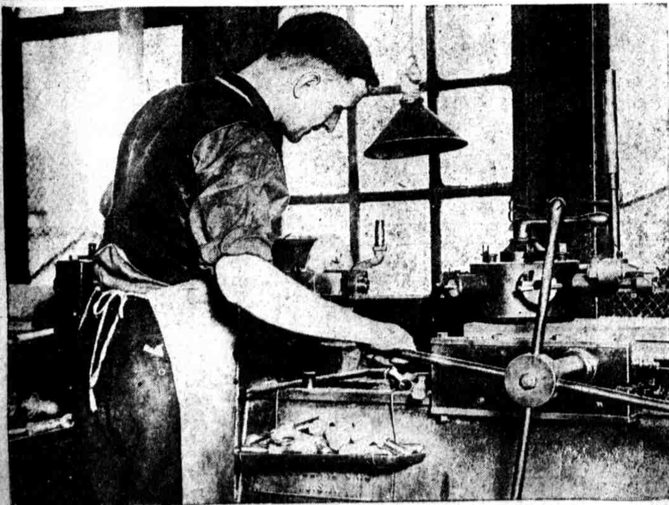
THREADING and putting seat on swan-neck faucets with a turret lathe at Thomas Savill's Sons, Thirteenth and Wallace streets. The operator, William Zerweck, of 2244 North Carlisle street, threads about 350 faucets a day.
