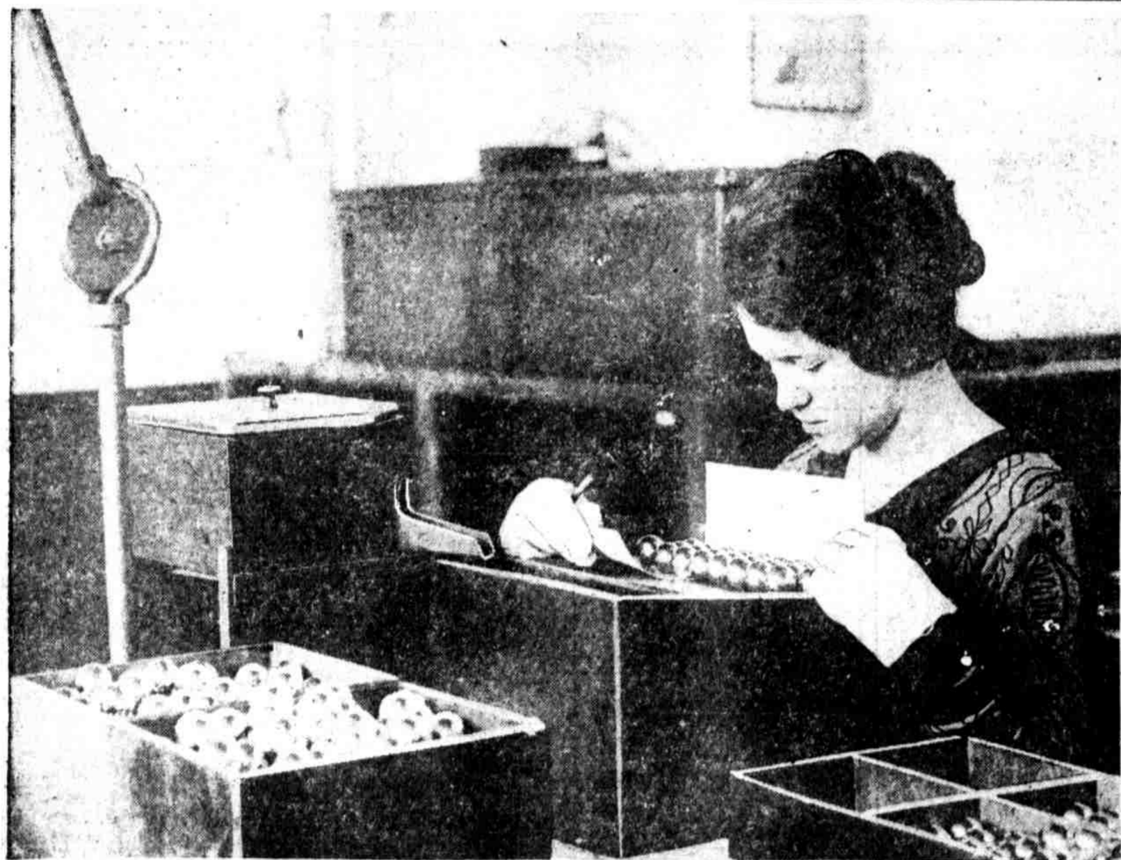
FINAL INSPECTION OF THE STEEL BALLS, manufactured by the Atlas Ball Co. at their factory, Fourth street and Glenwood avenue. Miss Rosetta Parker, 2332 North Van Pelt street, is seeing that the finished steel balls have no surface defects.
