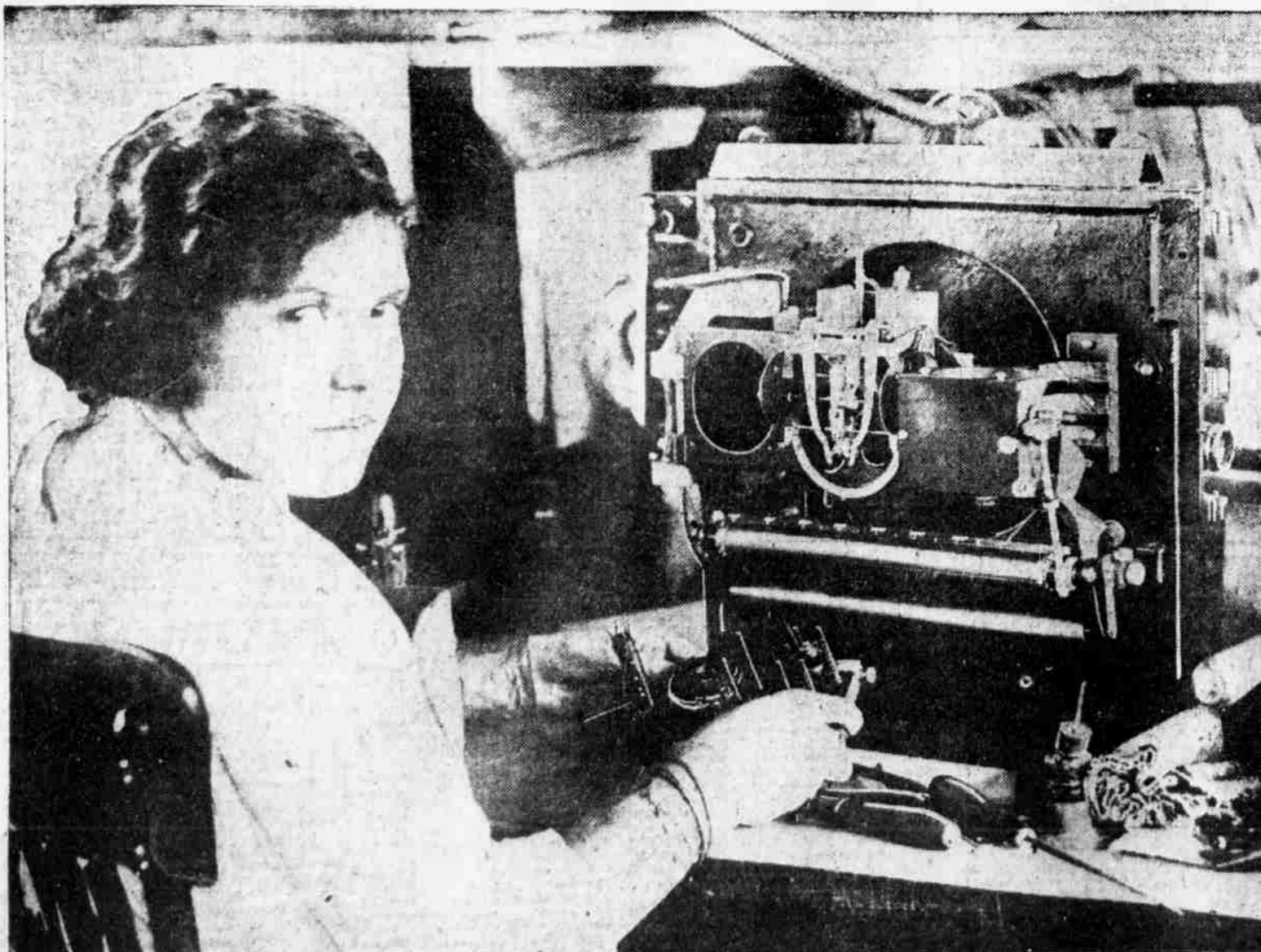
Miss Wilhemia Binder, of 3760 North Fifteenth street, is shown making electric connections on a potentiometer pyrometer recorder used for measurement of high temperatures. Its capacity for recording heat is 2500 degrees Fahrenheit. These recorders, used for automobile steel testing, are made by Leeds & Northrup, 4901 Stenton avenue.
