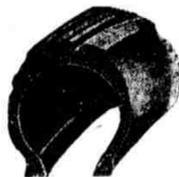
This is a "buckling" of the fabric under pressure—it is pinched up into the cushion and tread stock. And as this is the point of greatest strain on a tire, where the full load is concentrated, the casing soon gives way—and blows out.
