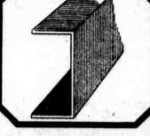
Cross section showing heavy construction of Fulton frame. Cold rolled steel 3/16<sup>4</sup> thick, 5<sup>1</sup>4<sup>4</sup> deep with a 2<sup>1</sup>4<sup>8</sup> angle.
