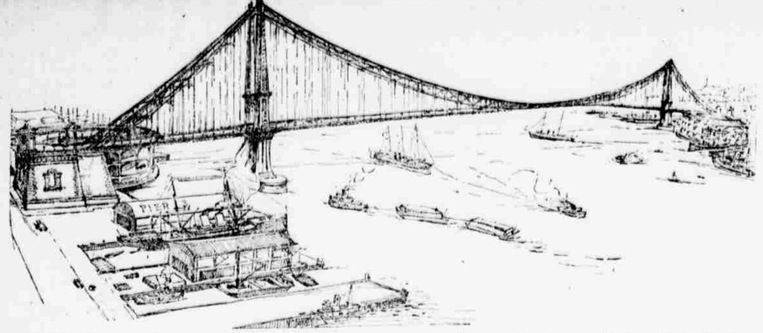
Engineers acting for the Pennsylvania and New Jersey bridge commissions have drawn up plans for the world's longest suspension span to connect Philadelphia and Camden. The bridge, which would cost between $10,000,000 and $12,000,000 to construct, would be 115 feet wide, have four railway tracks, two promenades and two roadways.
