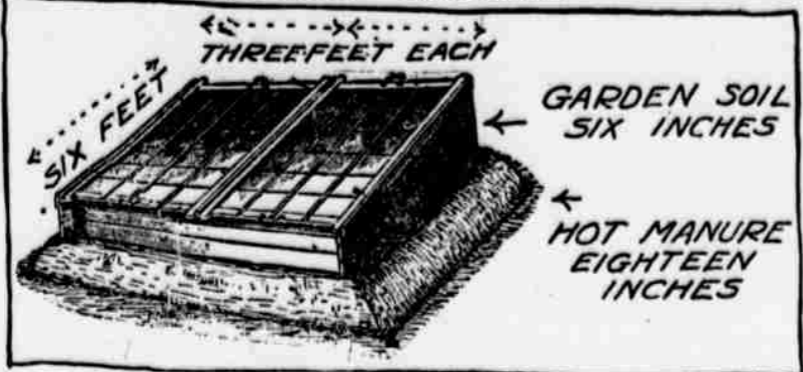
CONSTRUCTION OF HOTBED
