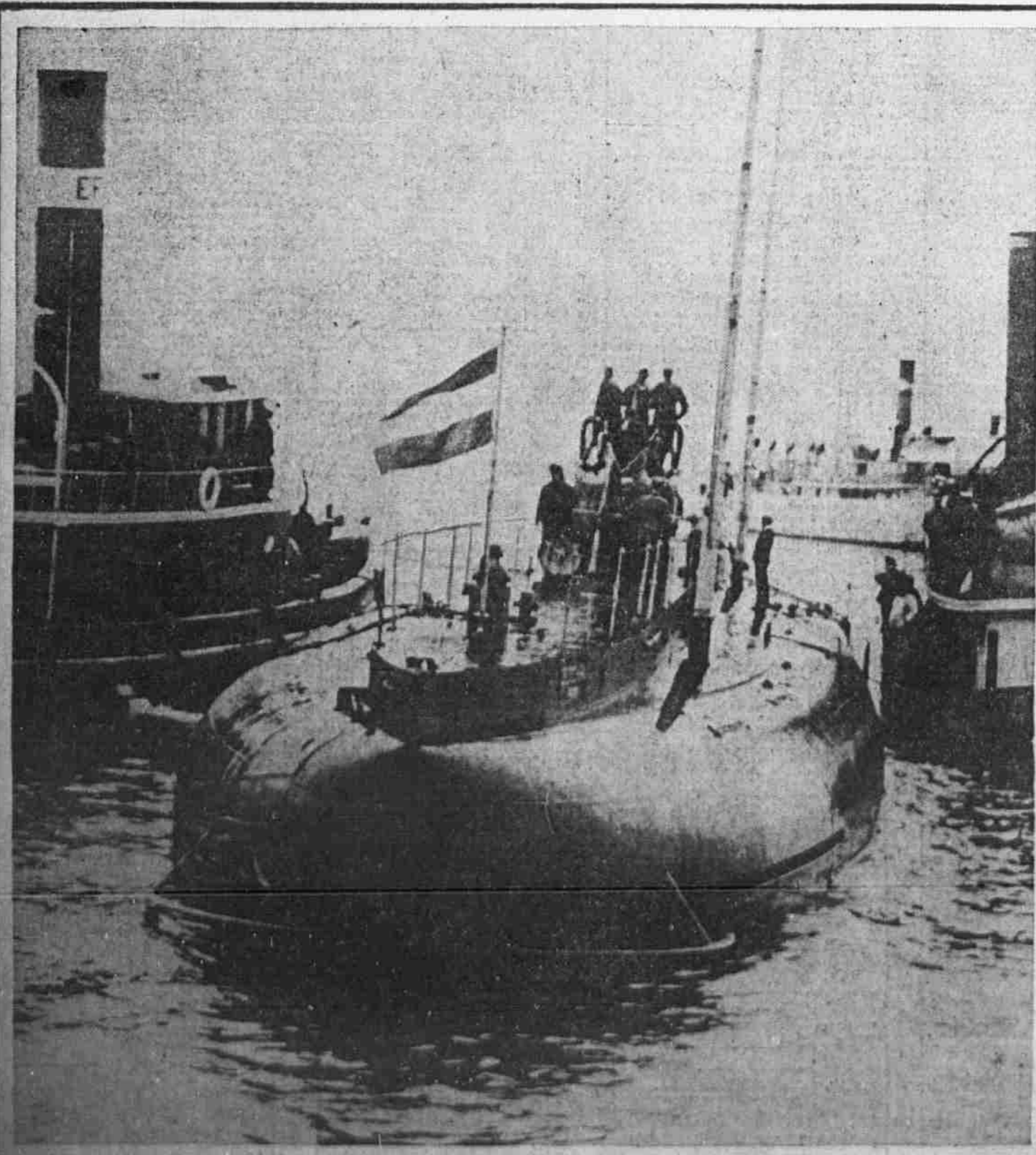
STERN VIEW OF THE NEW SUBMARINE MERCHANTMAN, SHOWING HER BULGING UNDERWATER BODY, AND HER COMMANDER, CAPTAIN KOENIG This view of the craft shows how she is built so as to provide roomy cargo space beneath her narrow superstructure. She is in tow of the tugs Elco and Timmins. The other picture shows her skipper, in his naval cap and sou'wester, standing beside Captain Hinsch, of the Baltimore company organized to handle the Deutschland's cargo. Photos by Harry Hood, Staff Photographers.
