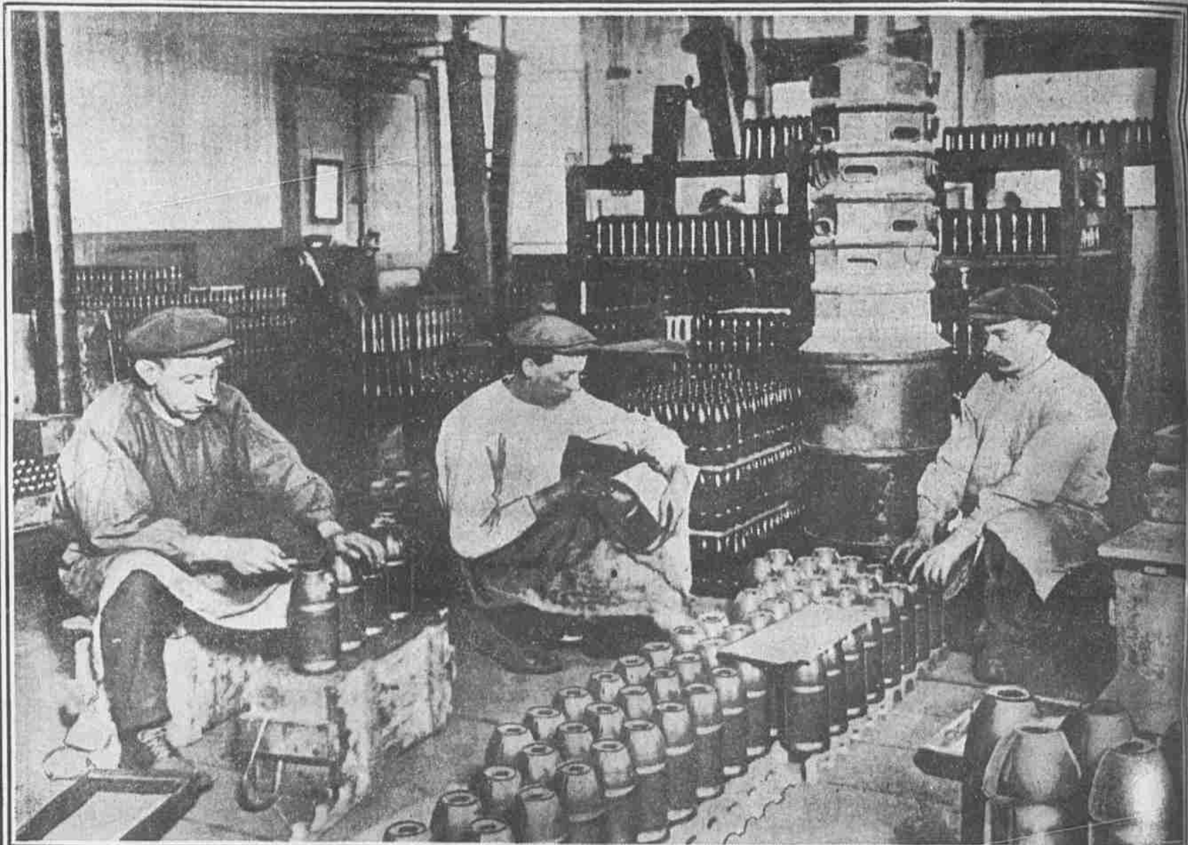
PREPARING THE SHELLS FOR THEIR EXPLODERS The noses of some types of shells are hollowed out for the reception of caps or fuses, which cause an explosion at the moment of striking. The missiles are then sorted and made ready for packing.
