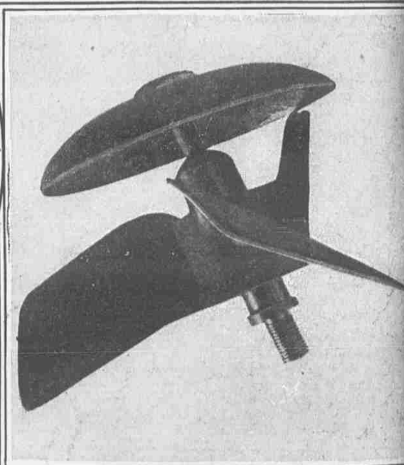
PROPELLERS FITTED TO GERMANY'S AERO MISSILES This small propeller, with three three-inch blades, was found attached to an exploded bomb dropped on a field at Beldington, Northumberland, England, from a German Zeppelin in a recent raid.
