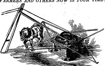
HAINES' IMPROVED LIGHT DRAUGHT HORSE POWER. HE above cut represents the plan of my Horse Power, and the manner in which the Strap passo out over the Horse's back. The Power is very simple in its construction and is arranged to su
