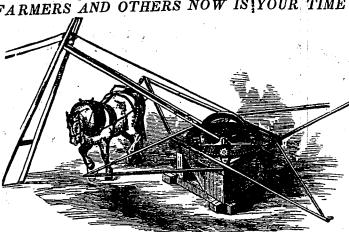
HAINES' IMPROVED LIGHT DRAUGHT HORSE POWER. the above cut represents the plan of my Horse Power, and the manner in which the Strap pout over the Horse's back. The Power is very simple in its construction and is arranged to er 1, 2, 3 or 4 Horses.
