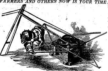
HAINES' IMPROVED LIGHT DRAUGHT HORSE POWER. HE above cut represents the plan of my Horse Power, and the manner in which the Strap passe out over the Horse's back. The Power is, very simple in its construction and is arranged to sui In out over the Horse's back. The Power is, very simple in its construction and is arranged to suither 1, 2, 3 or 4 Horses.
