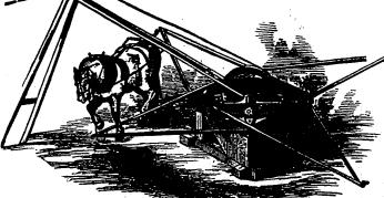
HAINES IMPROVED LIGHT DRAUGHT HORSE POWER. HE above cut represents the plan of my Horse Power, and the manner in which the Strap passes out over the Horse's back. The Power is very simple in its construction and is arranged to su either 1, 2, 3 or 4 Horses.
