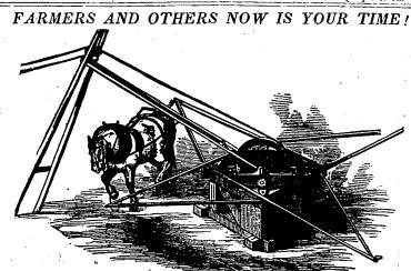
HAINES' IMPROVED LIGHT DRAUGHT HORSE POWER. THE above cut represents the plan of my Horse Power, and the manner in which the Strap passes out over the Horse's back. The Power is very simple in its construction and is arranged to suit It is particularly adapted to the use of Threshing Machines. I will dispose of STATE OR COUNTY
