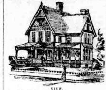
by the National Building Plan associa tion, Detroit. It may have either brick or stone foundation and a 6 foot 6 inch cellar. The first story is 10 feet high, and con tains a hall which is 20 feet long by 7 feet wide; a parlor measuring 14 by 17 feet; a
