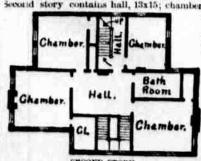
SECOND STORY. with fireplace), 14x15; chamber, 14x14; chamber, 10x14; chamber, 13x15; closet off such chamber; bathroom, 7x11.6. Estimated cost of building, \$8,000.
