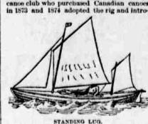
duced it into the States. It has gained con siderable favor since, one reason undoubted ly being that there are but two lines to each sail-the halliard and the sheet. The sprit boom keeps the sail very flat, thus making it especially effective in windward work. The
