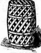
A VENTILATED BARREL The body of the barrel is formed of two or more layers or thicknesses of the splints crossing each other diagonally, the splints being nailed to each other and to the supporting hoops, as many hoops being employed as are deemed necessary or desirable. The head and bottom of or desirable. The head and bottom of the barrel may be put in in any desired
