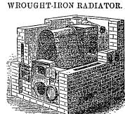
riveted together, the only sure prevention against the escape of Gas or Dust. They are easily managed, without-any dampers. The Patent Radiator avoids the use and annoyances of drums, and is permanently attached to the Heater. This is the most durable, simple, economic ul, and popular Heating Apparatus ever offered for sale They are all guaranteed.
