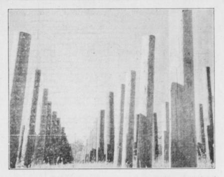
One of the most unusual "plantations" in the world is to be found at Chester, N. J., where the Bell Telephone Laboratories carries on research work to determine what types of telephone poles are the safest, the most economical and give the best service. Hundreds of poles of various kinds of wood treated with preservatives are planted on this proving ground and examined at regular intervals during their life-time.
