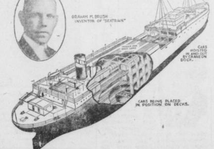
hours 100 loaded freight cars will be | "Seatrain" expands the freight put aboard; the ship will have swal- container idea to the scale of the lowed a freight train a mile long, freight car. Eliminating packing expense, it also does away with loss and be ready for sea.
