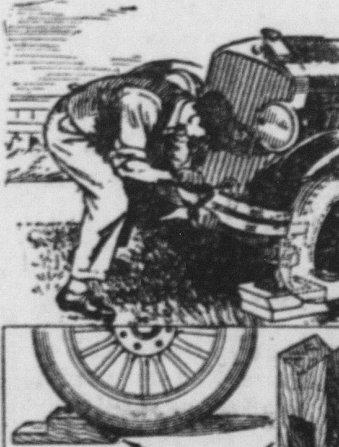
BLOCKS BOLTED TOGETHER FOR A STAND FOR CENTER OF FRONT AXLE
