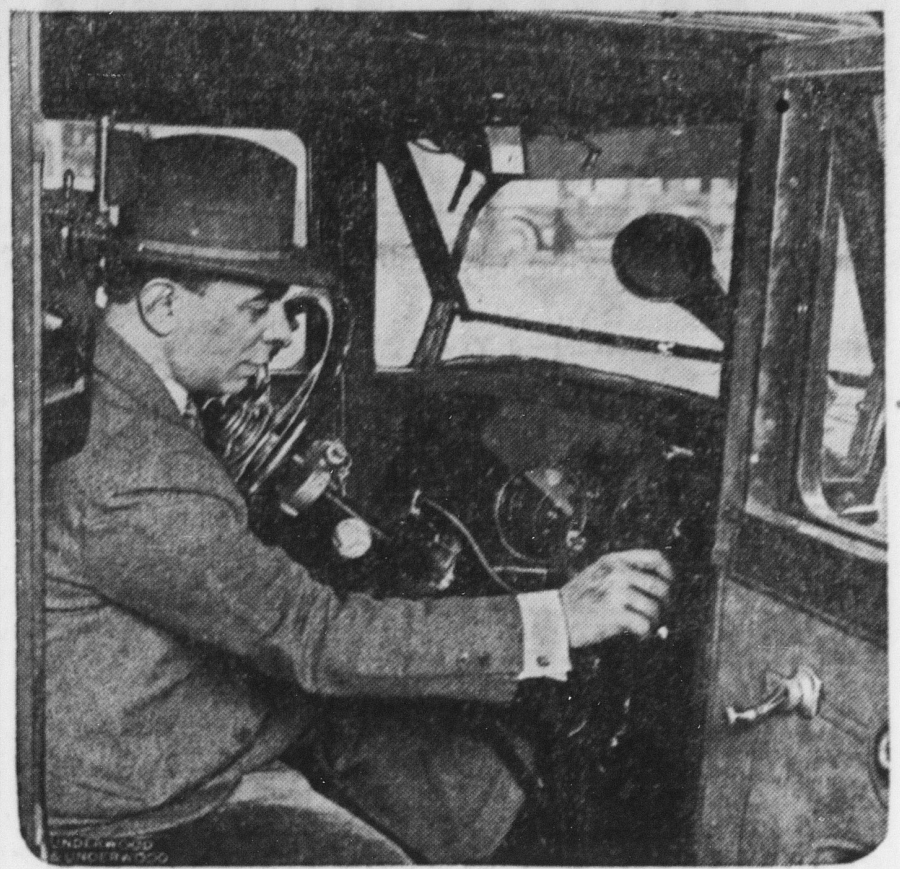
One of Chicago's privately owned taxi cab lines now entertains its patrons by radio. Our photo shows one of the taxis on the streets of Chicago equipped with a two-dial set and loud speaker. At the extreme right on the dash board are the two dials, while the loud speaker is shown on the glass windshield.
