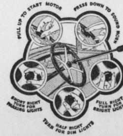
A single button, conveniently located in the center of the steering wheel, controls all funetions of starting the motor, operating the lights and sounding the horn. This does away with all troublesome foot fumbling for the starting button. It also avoids changing from the comfortable driving position to reach a light switch on the dash. With the new "Finger-Tip Control," you can at all times keep your hands on the wheel and your eyes on the road-an important aid to safety.
