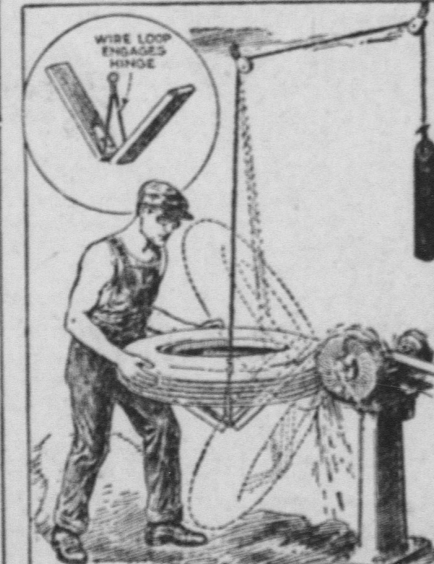
Handy Support for Holding Heavy Tires Against Buffing Wheel Eliminates Unnecessary Work.
