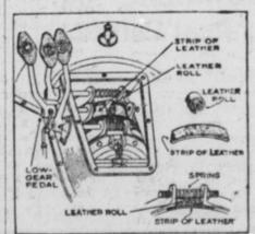
Strips of Leather, or Heavy Canvas, Make It Possible to Get the Light Automobile Into "High" When the Low-Gear Friction Band Burns Out.
