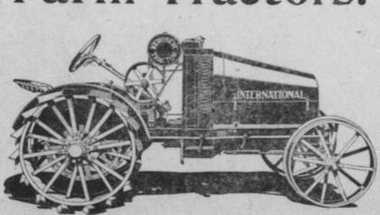
The International Harvester Co.'s 8-16 4-cylinder kerosene burner Tractor can plow on land or in the furrow.
