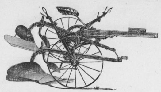
It plows the same depth the whole day long; sticks to the ground in stormy soil; can be well handled on rocky hillsides. It leaves no deep furrows to wash; will throw the soil up hill better than any other plow made; it is strong enough to do its work, yet not clumsy. Made for two or three horses.
