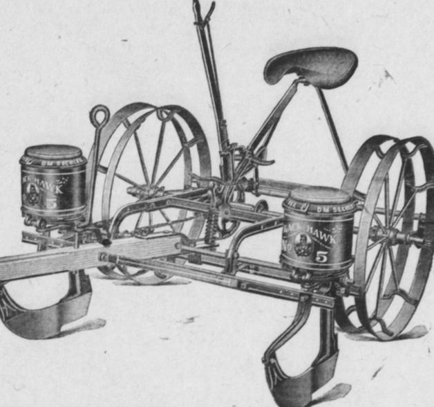
Adjustment, from 3 feet to 3 feet 8 inches. Wheels, 13 0 inches; open, concave or flat, as desired. Planter regularly furnished with tongue, and 5 sets of seed plates. With or without fertilizer attachment. When specified, this drill will be furnished adjusted, 2 feet 4 inches and 3 feet 4 inches to 4 feet.
