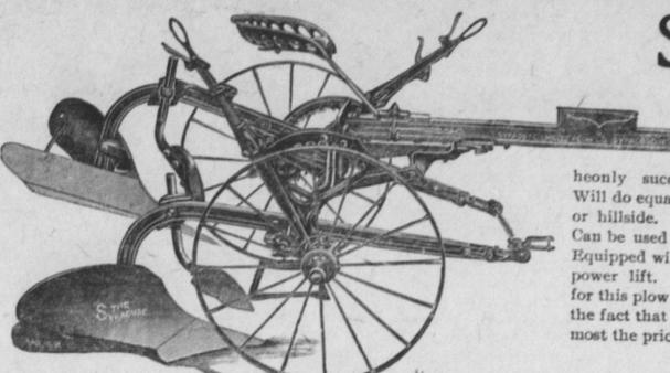
heonly successful hillside sulky made. Will do equally good work on level land or hillside. No dead or back furrows. Can be used with two or three horses. Equipped with foot trip which operates power lift. The best recommendation for this plow is the man who uses it, and the fact that at public sales it sold at almost the price of a new one.
